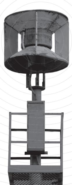
removal. For *War of the Worlds*, three downtown sirens were completely refurbished – the siren "heads" were detached, and old rusted and rotting parts were removed and replaced with new Meyer Sound speakers for the performance.
